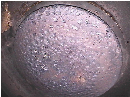
图 1 排气门头上沉积物形貌 Fig. 1 Morphology of sediment on exhaust valve head
